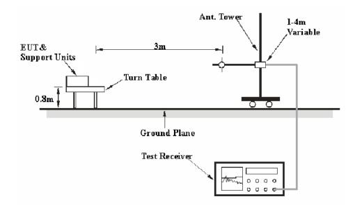
The radiated emission tests were performed in the 3 meters chamber test site, using the setup accordance with the ANSI C63.4-2009. The related limit was specified in FCC Part 15B.
