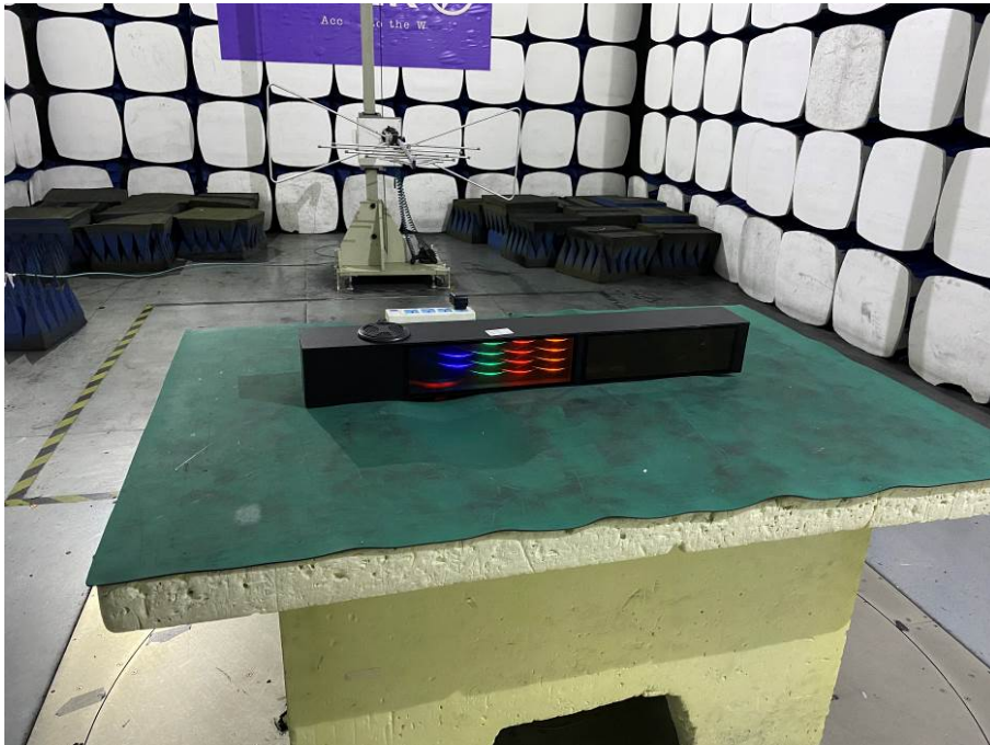
Spurious Emission Test Setup (Below 1GHz)
