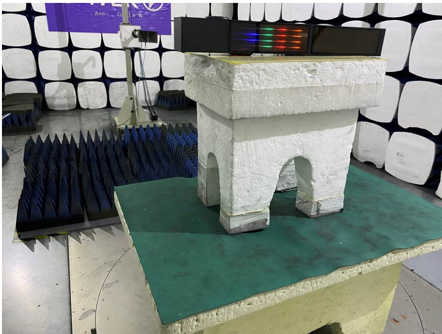
Spurious Emission Test Setup (Above 1GHz)
