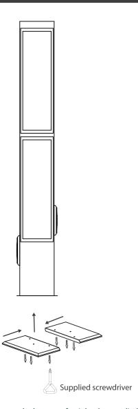
Assembly the two wooden bases to the bottom of unit by the supplied assembly screws and screwdriver as the illustrated above.
