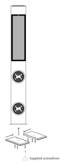
Assembly the two wooden bases to the bottom of unit by the supplied assembly screws and screwdriver as the illustrated above.
