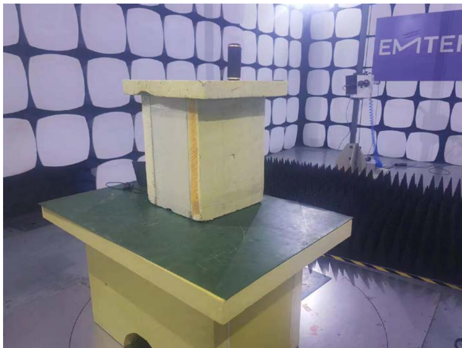
Spurious Emission Test Setup (Above 1GHz)
