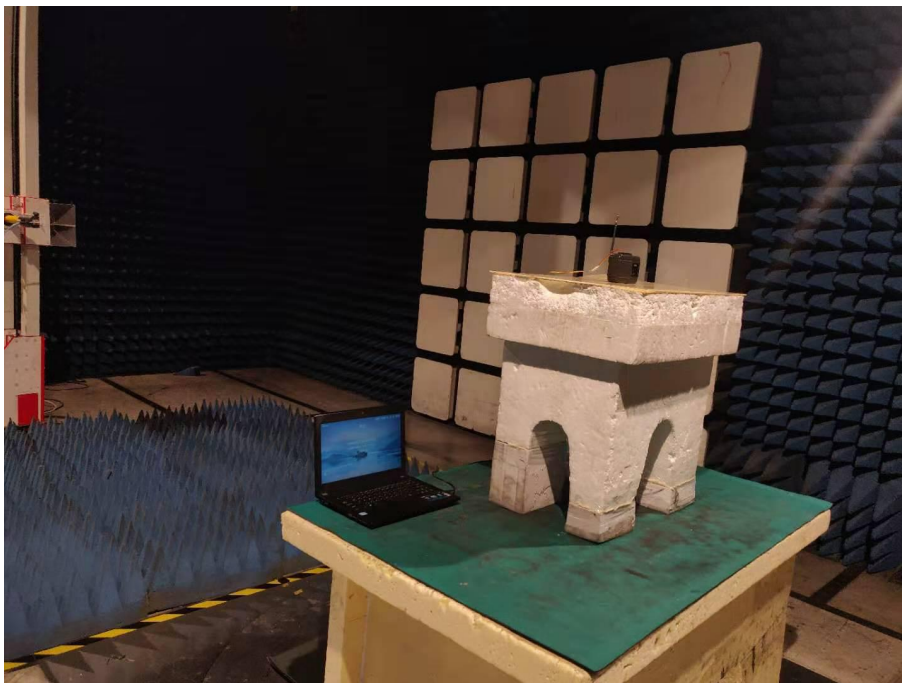
Spurious Emission Test Setup (Above 1GHz)
