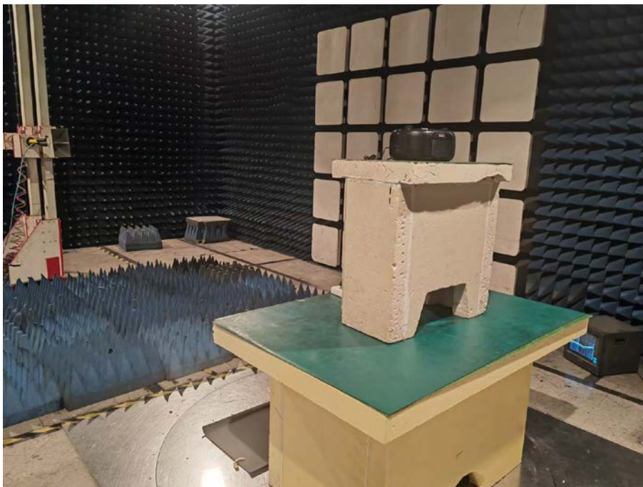
Spurious Emission Test Setup (Above 1GHz)
