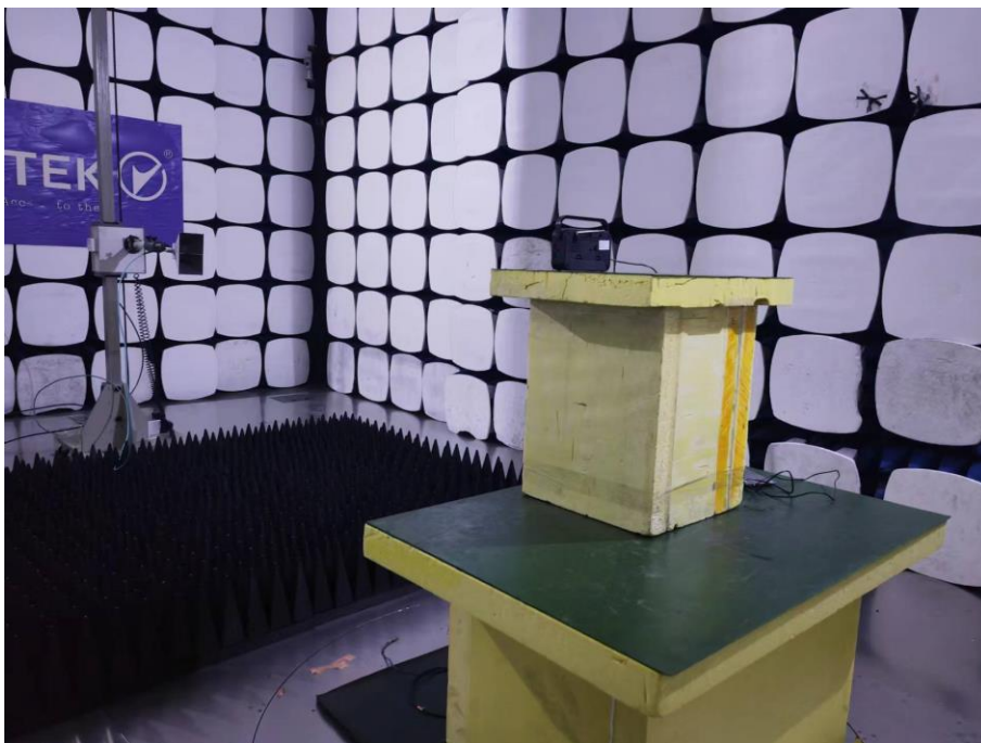
Spurious Emission Test Setup (Above 1GHz)
