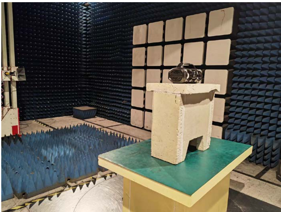
Spurious Emission Test Setup (Above 1GHz)
