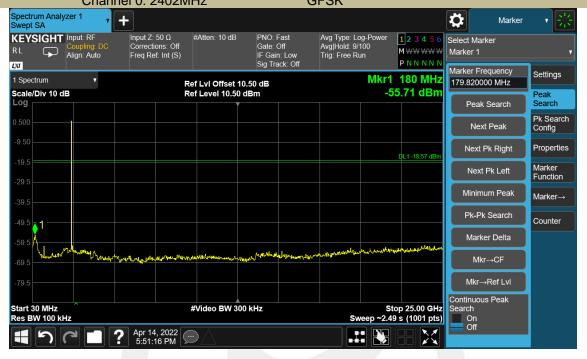
Test Model Maximum Conduceted Level RBW=100kHz
