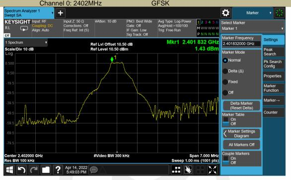
Test Model Band-edge Conducted Emissions
