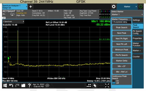
Test Model Maximum Conduceted Level RBW=100kHz
