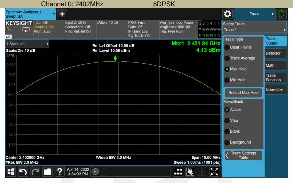
Test Model Maximum Peak Conducted Output Power
