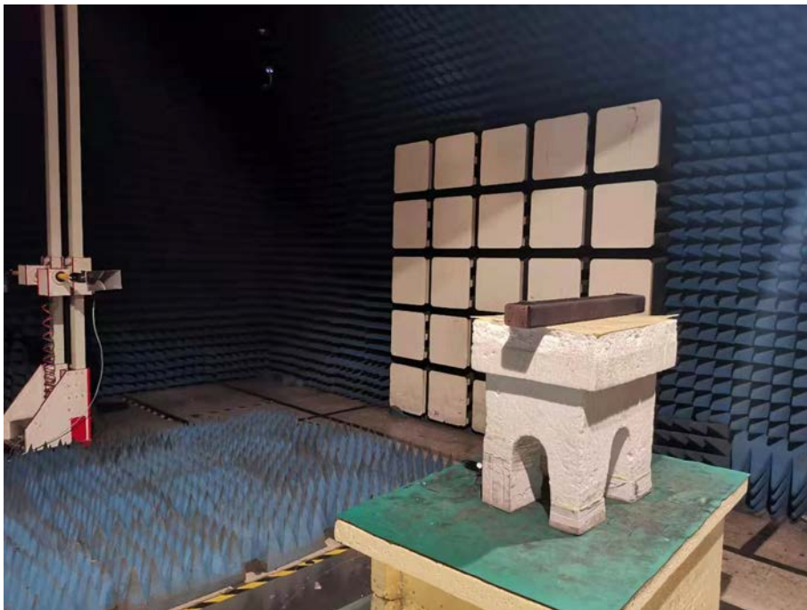
Spurious Emission Test Setup (Above 1GHz)
