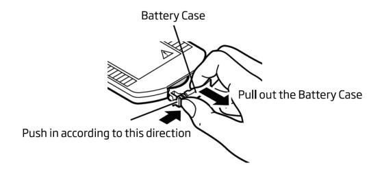
Replace the battery by a new CR2025 size battery. When inserting the battery, be sure to do so in the proper direction as shown below.
