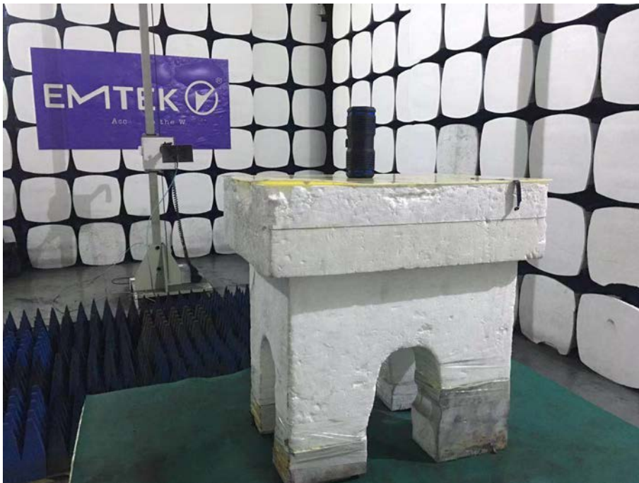
Spurious Emission Test Setup (Above 1GHz):
