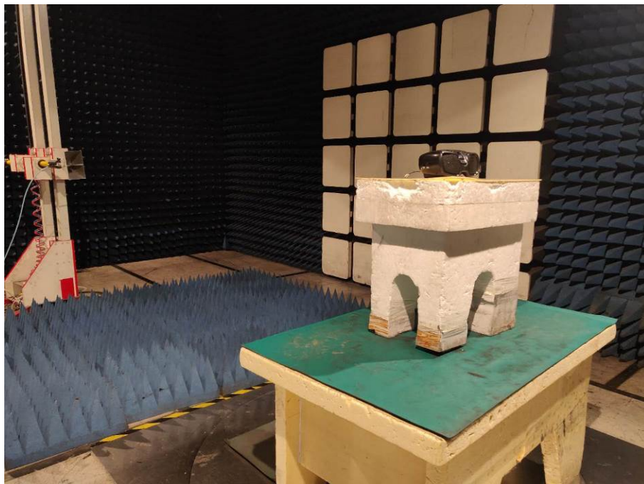
Spurious Emission Test Setup (Above 1GHz)
