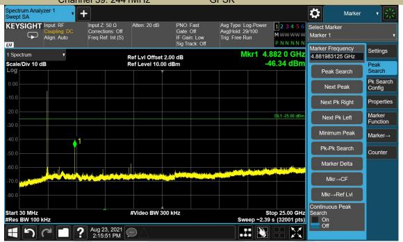
Test Model Maximum Conduceted Level RBW=100kHz
