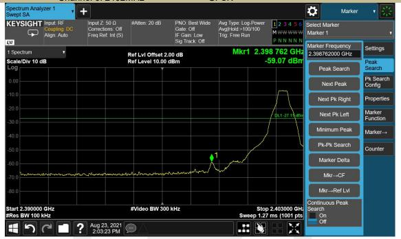
Maximum Conduceted Level RBW=100kHz
