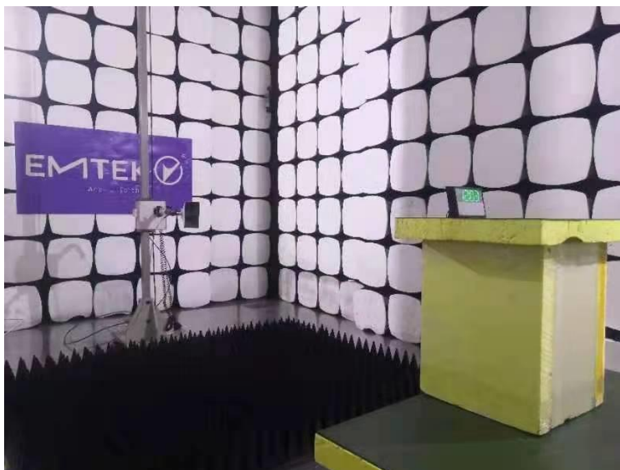
Spurious Emission Test Setup (Above 1GHz)
