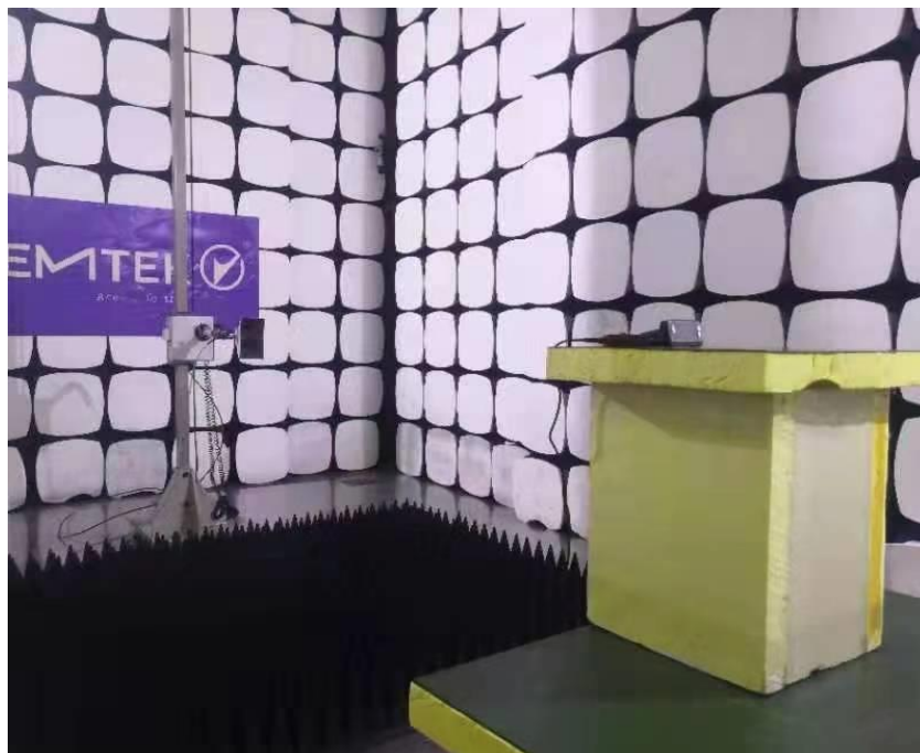
Spurious Emission Test Setup (Above 1GHz)
