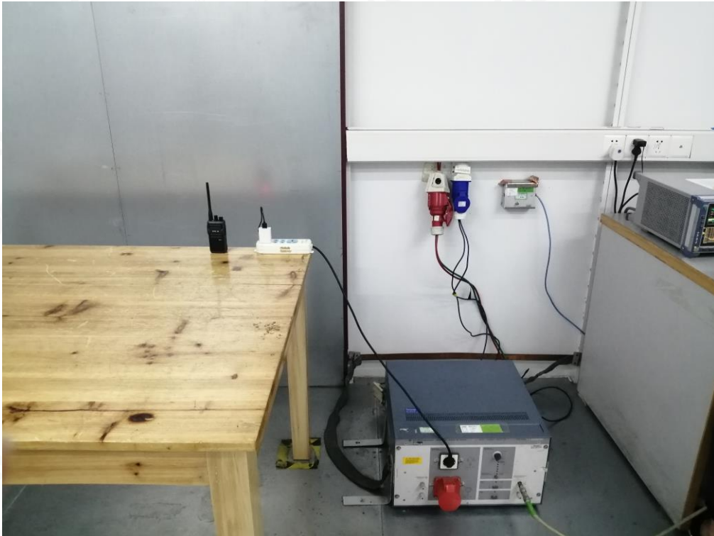
RADIATED EMISSION TEST SETUP-BELOW 1GHZ
