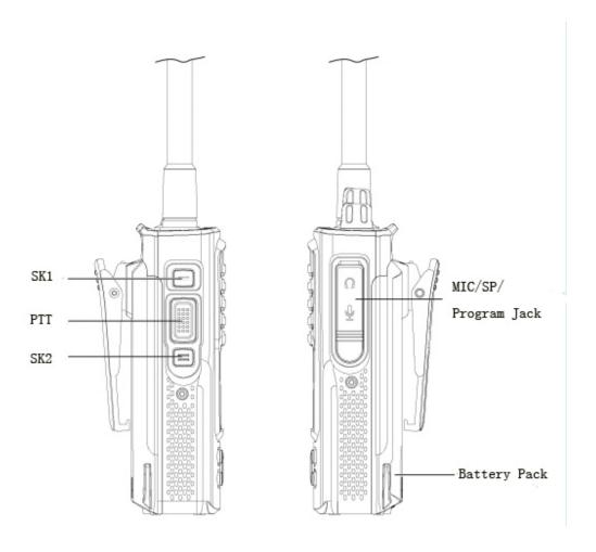
**Notice**: Either Long-press or Short-press of Side-key 1/ Side-key 2/ Side-key 3 can be set by program software for the following functions:
