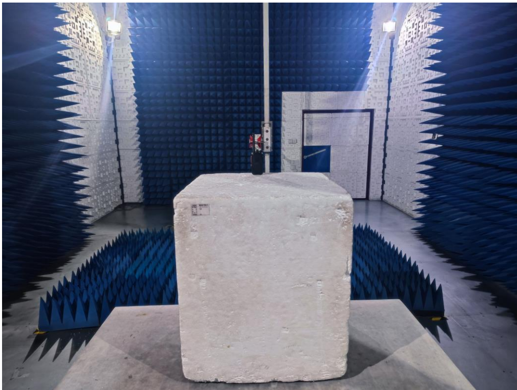
RADIATED EMISSION TEST SETUP ABOVE 1GHz
