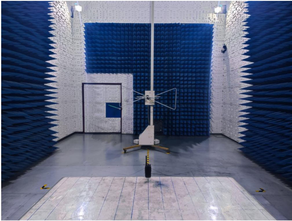
RADIATED EMISSION TEST SETUP ABOVE 1GHz
