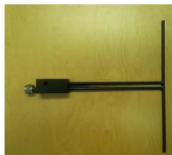
Figure 1 – MVG COMOSAR Validation Dipole
