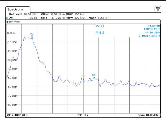
4.5 Out of Band Radiated Emissions (for emissions in 4.4 above that are less than 20dB below carrier), FCC Rule 15.247(d):
