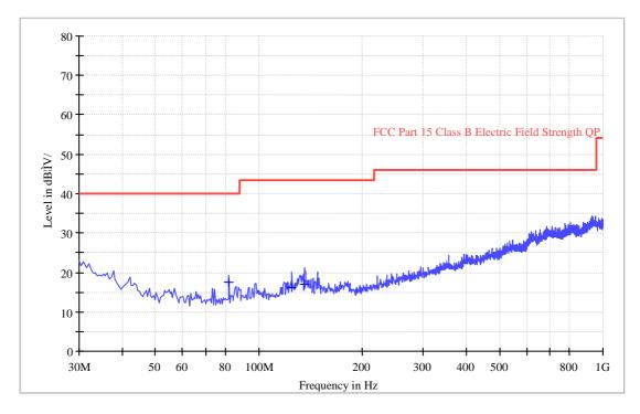
Applicant: S&O ELECTRONICS (MALAYSIA) SDN. BHD. Date of Test: April 9, 2016 Model: SA189AW Worst Case Operating Mode: Transmitting with AC/DC Adapter (2402MHz)
