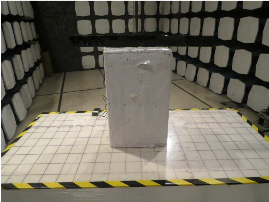
Front View of Radiated Emissions above 1GHz
