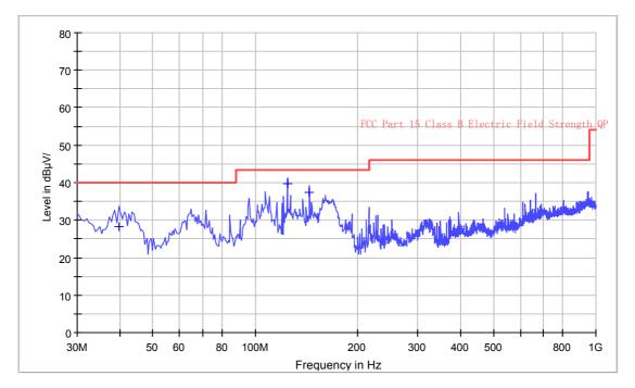
Applicant: S&O ELECTRONICS (MALAYSIA) SDN. BHD. Model: HT-SB38 Sample: 1/1 Worst Case Operating Mode: BT Link Modulation type: GFSK
