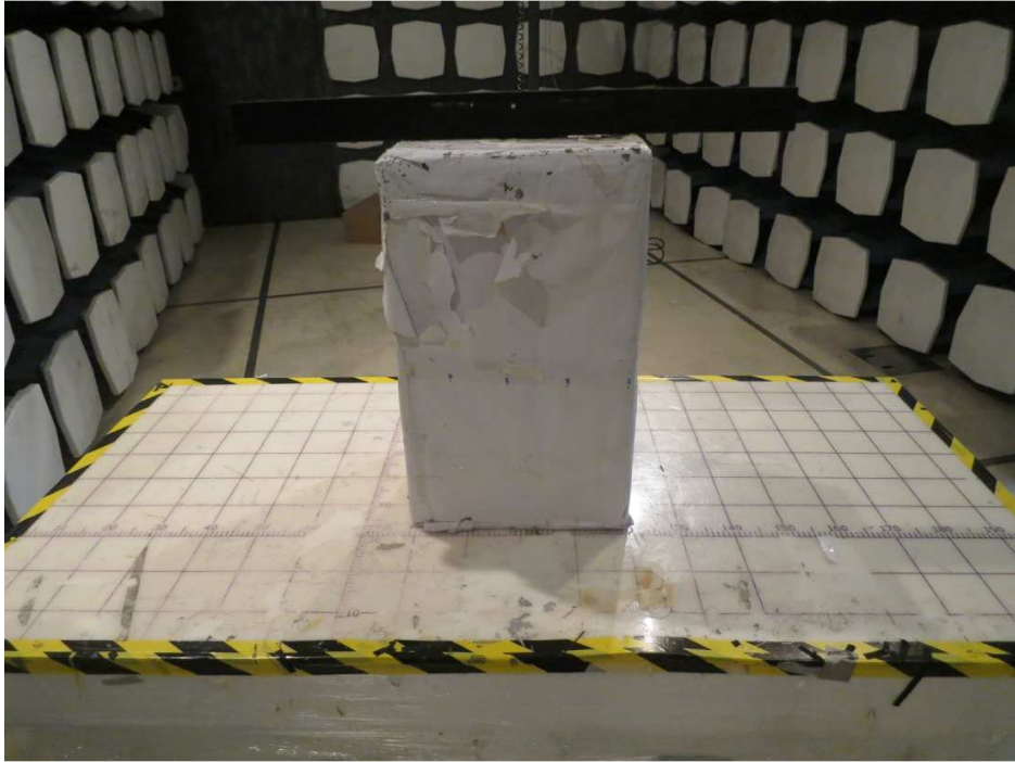
Front View of Radiated Emissions above 1GHz
