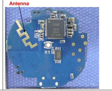
The antenna is PCB antenna. The best case gain of the antenna is 0dBi.
