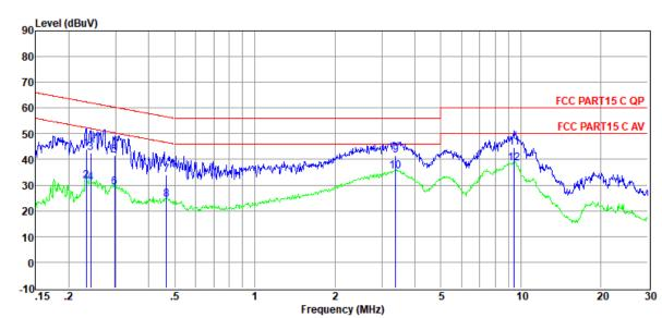
LISN Cable Pulse Result Limit Over Factor Loss Limiter Limit Level Line
