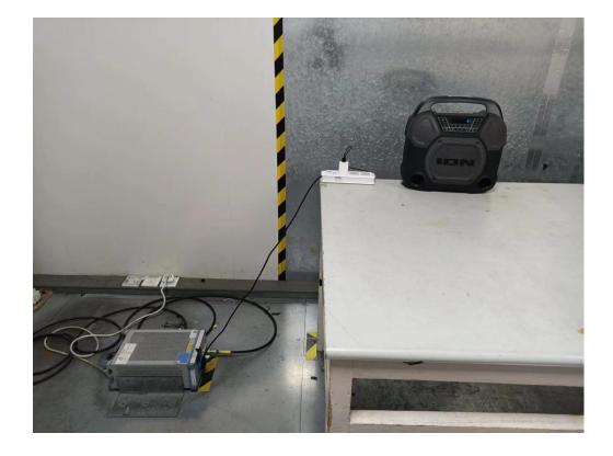
Radiated Test (30-1000 MHz)
