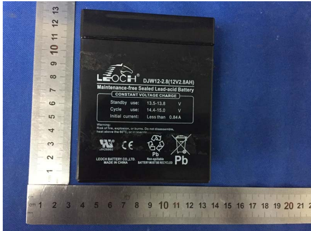
Built-in battery: DJW12-2.8
