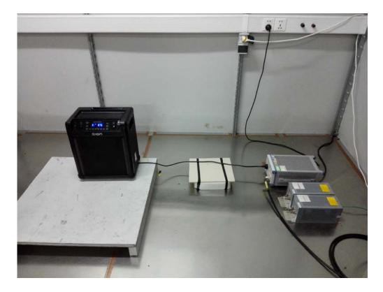
**1.2.** Photos of radiated emission test
