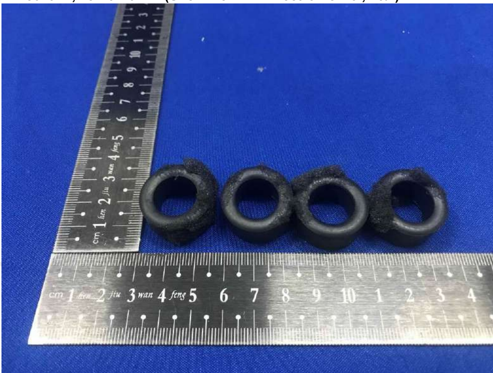
Magnet: V180194T, 28*13*16mm (ShenZhen VIIP Electronic Co., Ltd.)
