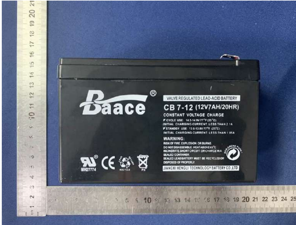
Battery Package: CB7-12 (JiangXi HengLi Battery Technology Co., Ltd)
