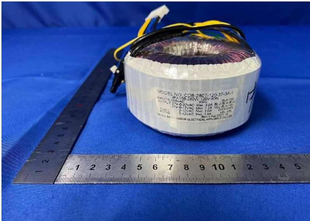
Mains linear transformer (YUYAO ZHONG CHI ELECTRIC ALAPPLIANCE. CO. LTD)
