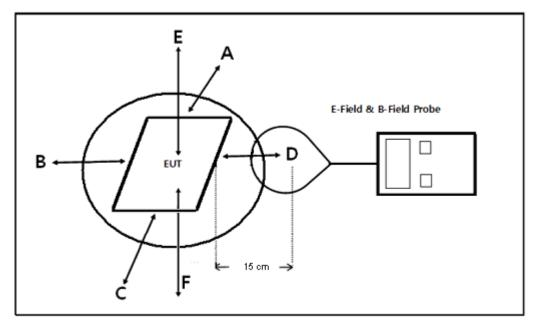
Note: Due to installation limitations no tests from the underside of the charging device (Test Position F) are required.
