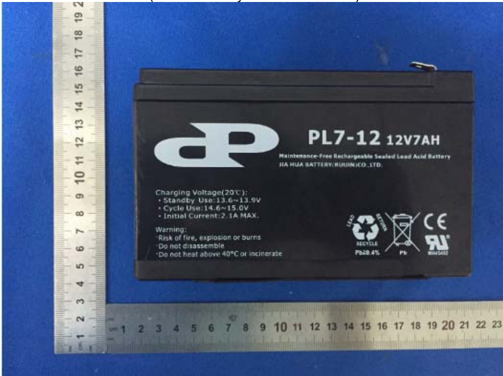
(Built-in Battery: Jia Hua / PL7-12)
