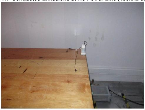
1.2 Radiated Spurious Emissions Test Setup
