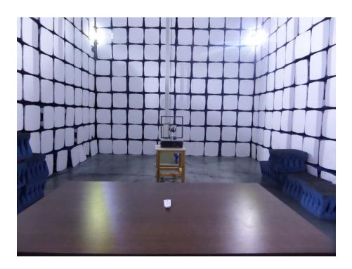
Radiation Emission Test Setup (30MHz to 1GHz)
