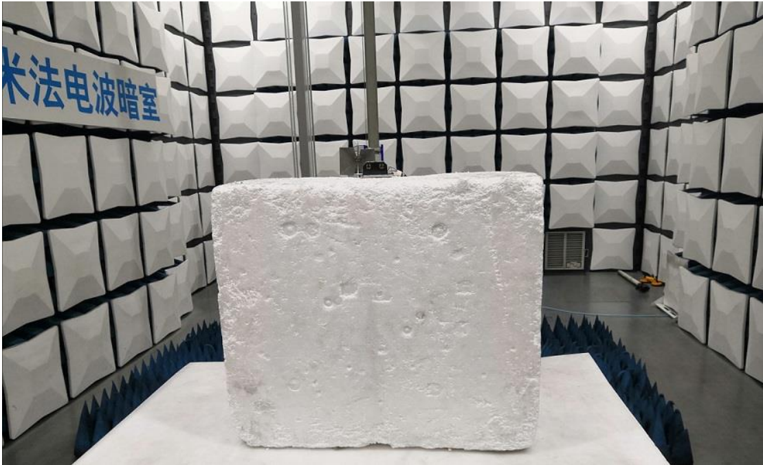
Radiated Emission test Above 1GHz
