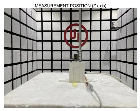
RADIATED RF MEASUREMENT SETUP (30MHz~1GHz)
