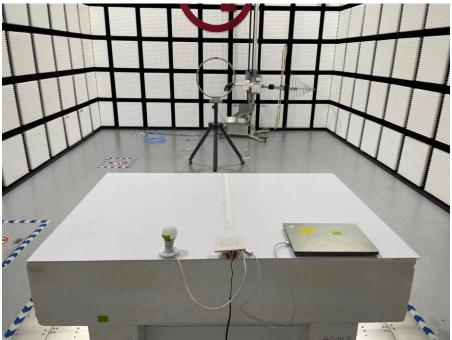
POWERLINE CONDUCTED EMISSIONS MEASUREMENT SETUP
