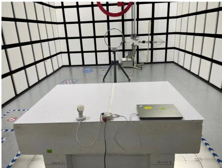
POWERLINE CONDUCTED EMISSIONS MEASUREMENT SETUP
