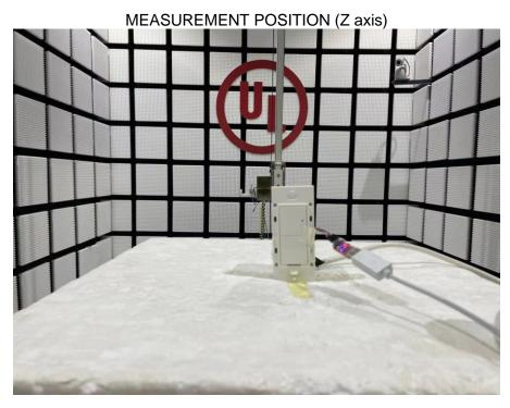
RADIATED RF MEASUREMENT SETUP (30MHz~1GHz)
