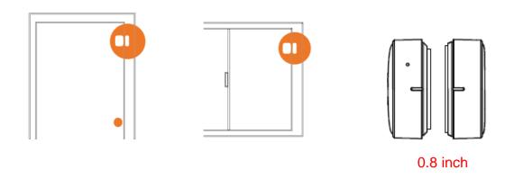
**Step 2:** Fix the bracket to door or window with either screws or adhesive tape for different surfaces.
