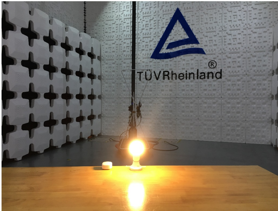
Photograph 3: Set-up for Radiated Emission, below 1GHz
