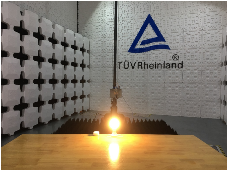
Photograph 4: Set-up for Radiated Emission, above 1GHz
