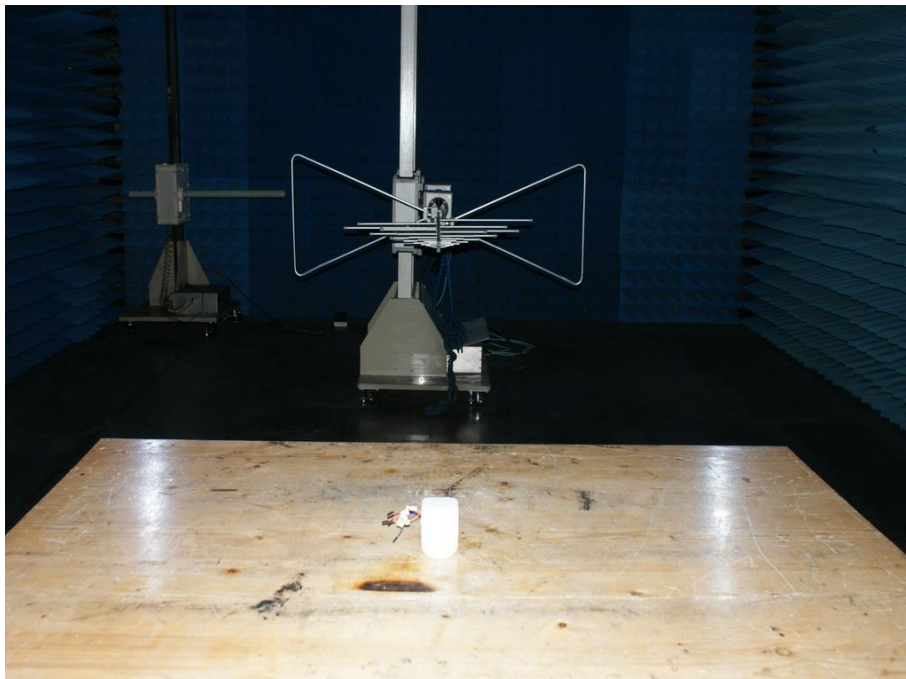
Photograph 2: Set-up for Radiated Spurious Emission, 30MHz - 1GHz
