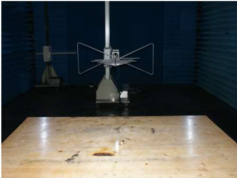
Photograph 2: Set-up for Radiated Spurious Emission, 30MHz - 1GHz
