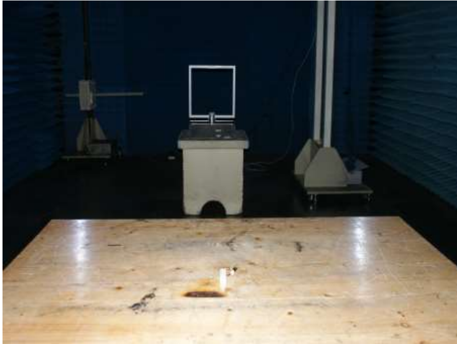
Photograph 1: Set-up for Radiated Spurious Emission, 9KHz - 30MHz
