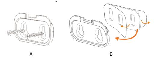
If you use adhesive tape, please clean the mounting surface with a suitable degreaser agent. Please note that some surfaces may be unsuitable for mounting using the adhesive tape. **Step 2:** Hang the keypad on the bracket.
