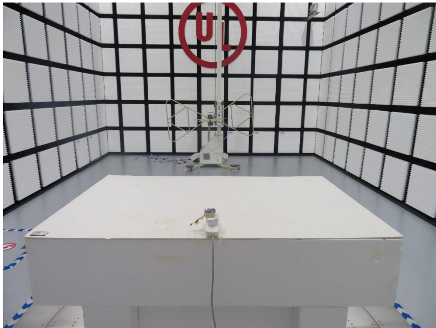
RADIATED RF MEASUREMENT SETUP (30MHz~1GHz)
