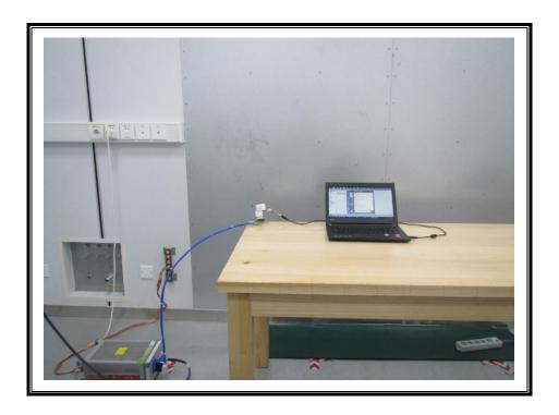
RADIATED RF MEASUREMENT SETUP (Below 30MHz)
