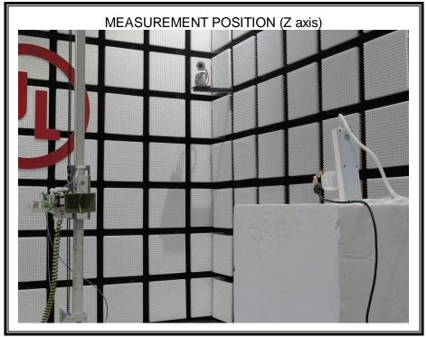
RADIATED RF MEASUREMENT SETUP (30MHz~1GHz)
