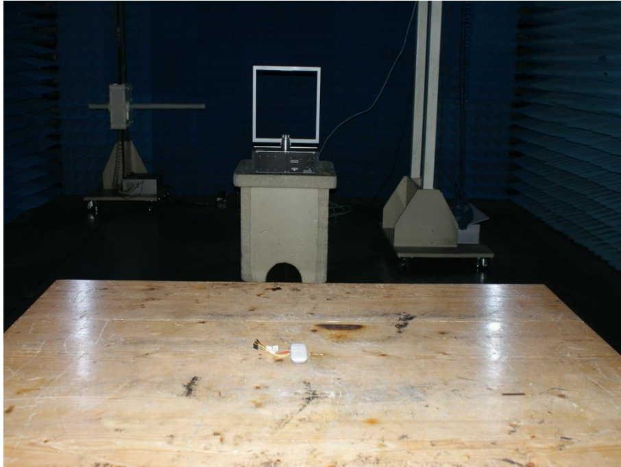
Photograph 1: Set-up for Radiated Spurious Emission, 9KHz - 30MHz
