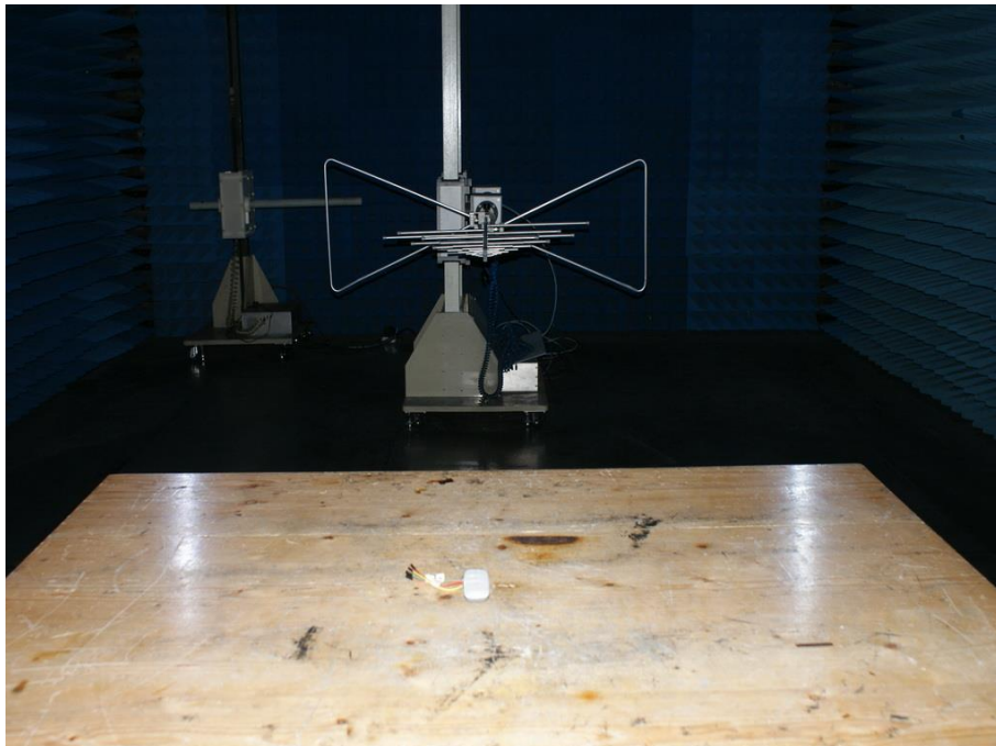
Photograph 2: Set-up for Radiated Spurious Emission, 30MHz - 1GHz
