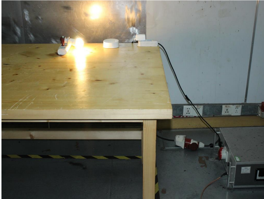
Photograph 1: Set-up for Conducted Emission on AC Mains
