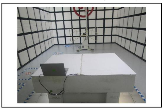
RADIATED RF MEASUREMENT SETUP (Below 30MHz)
